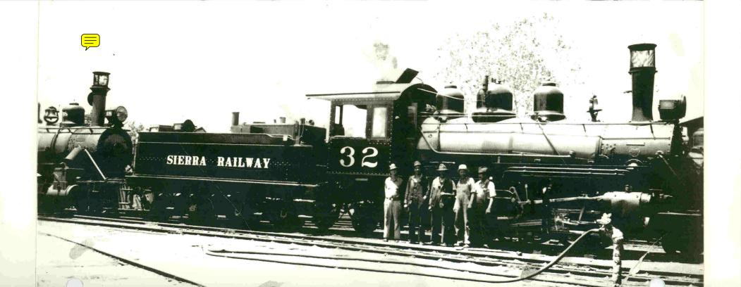
This locomotive was originally Sierra Railway No. 30. It was the regular Angels Branch locomotove from 1922, when it was built for use on that line, until the branch line was abandoned. When Howard Terminal Ry. purchased it from the Sierra Railway in 1937, workers removed the tender and added the saddle tank that rests on the boiler. Now this locomotive is at the Castro Point Railway Museum near Richmond, California.
